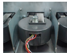
DCCT current sensor (in the PW3337)
